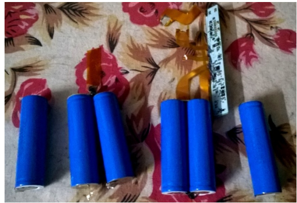
Six li-ion cells
