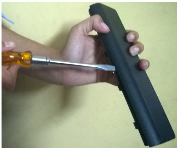
Finding the weak point to break the seal
